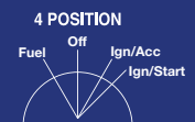
Key removable in Off position only, spring return to Ign/Acc position, spring return to Off from Fuel.
